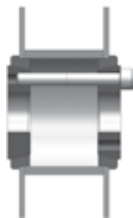
Applications that require spacing between thin end discs can be accommodated by extending the pilot surface through the end discs so that it engages a spacer and keeps the entire assembly aligned.
