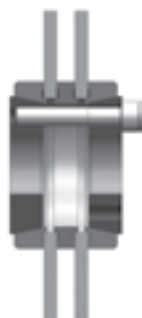
A double strand chain sprocket can be easily made by adding a spacer between two A-plate sprockets.
