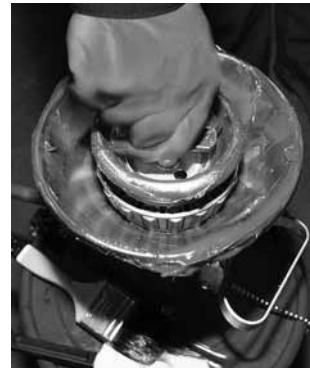
Fig. 24. Mechanical grease packer.
