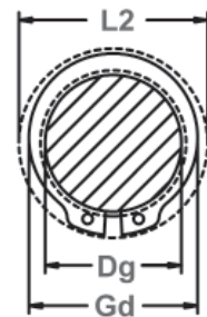
Clearance Diameter & Gaging Diameter Released in Groove
