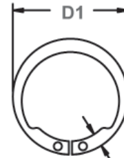
Measuring Free Diameter (Df) SHI Series Df = D1 - 2(S max)
